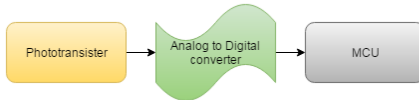
Figure 33 Detector Low Level Block Diagram
